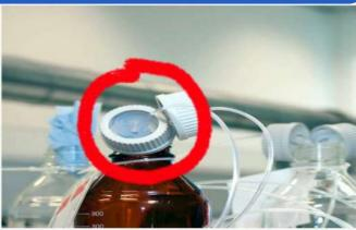
Solvent vapours are toxic and flammable. Especially during HPLC operation, multiple types of solvent reservoirs and fluid waste containers will raise the risk of health and environment damage if they are not properly tightened.
